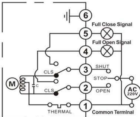
**A: ON/OFF Type with Light Indicator Signal Feedback**
