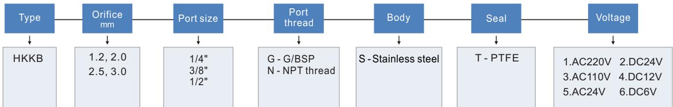
EXMAPLE: NC, 3.0MM ORIFICE, 1/4"G, STAINLESS STEEL BODY, PET SEAL, COIL S21B, AC220V, DIN
